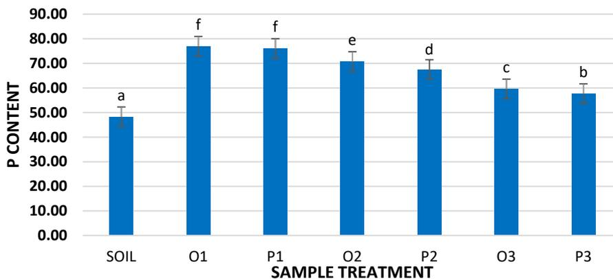
**Fig. 5:** The difference concentration of P (mg/L) for all sample treatments using spectrophotometry method in the presence of molybdovanadate reagent and tested in UV spectrophotometer at a wavelength of 400 - 450 nm. Tested values are significantly different at  $p \leq 0.05$  (one-way ANOVA)
