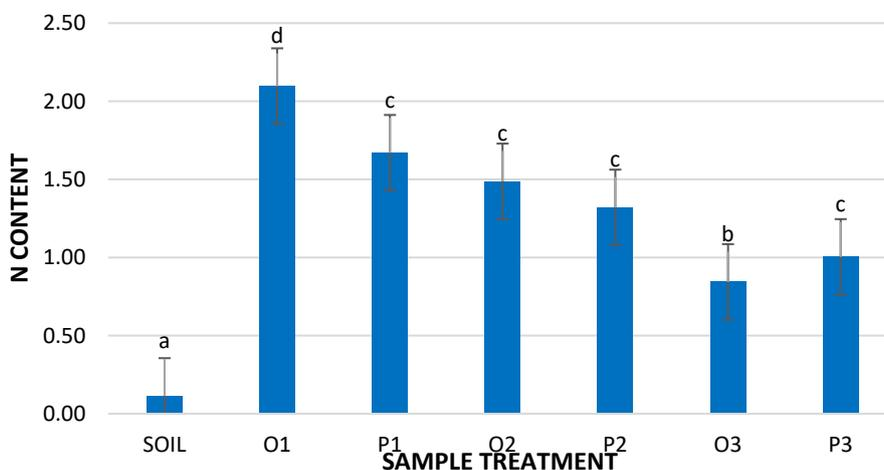
**Fig. 4:** The differences in N content in every sample treatment using the regular Kjeldahl digestion method. Tested values are significantly different at  $p \leq 0.05$  (one-way ANOVA)
