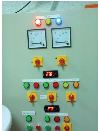
Figure 2: Environmental chamber main switch controller
