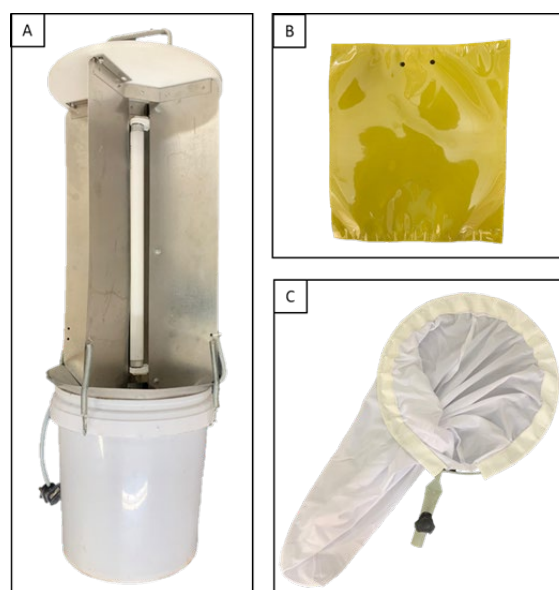
Figure 2: Sampling tools for the study; (A) bucket-light trap, (B) sticky trap and (C) sweep net.
