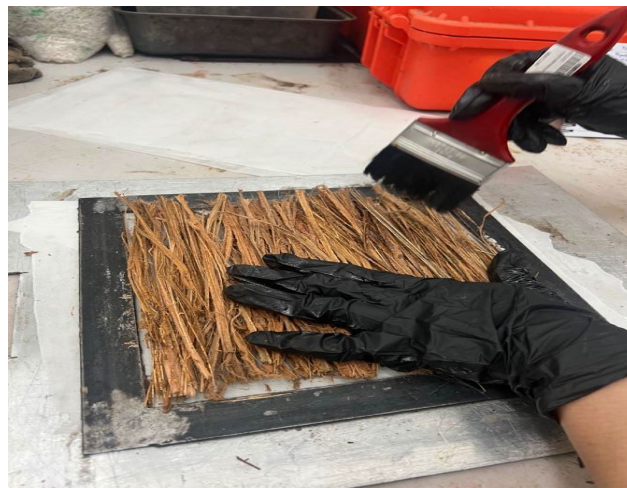
Figure 1: Adhesive coating process on the Nipah palm long fibres
