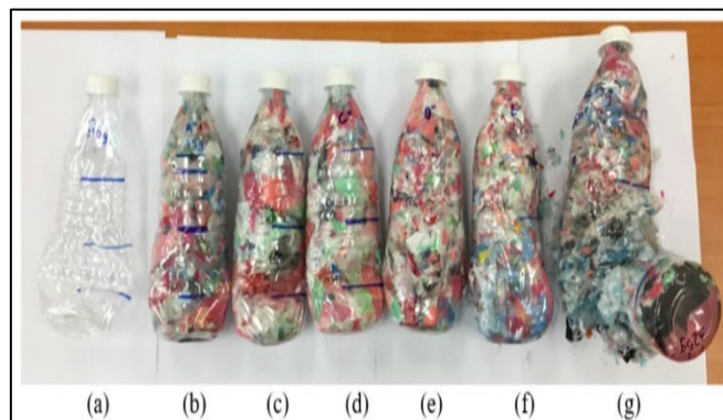
Figure 5: Ecobrick sample after flexural test: (a) Sample A, (b) Sample B, (c) Sample C, (d) Sample D, (e) Sample E, (f) Sample F, and (g) Sample G
