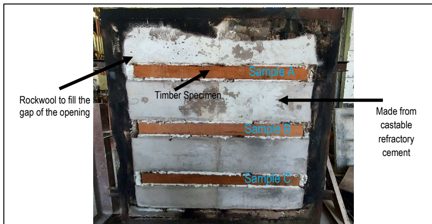
Figure 3. Frame used to place the specimens in position, with gaps filled using rock wool for insulation.
