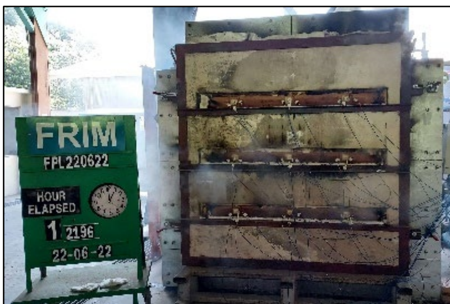
Figure 4. Specimens have been installed and ready for fire test
