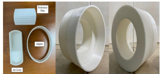
Figure 6: 3D printed samples for installation
