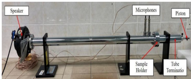
Figure 5: Impedance tube experimental setup
