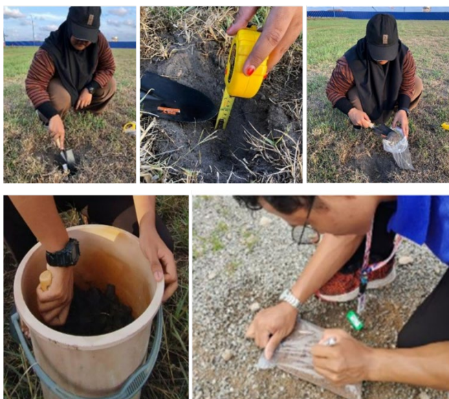
Figure 3: Procedures taking the soil samples – digging, measuring depth, mixing, and labelling
