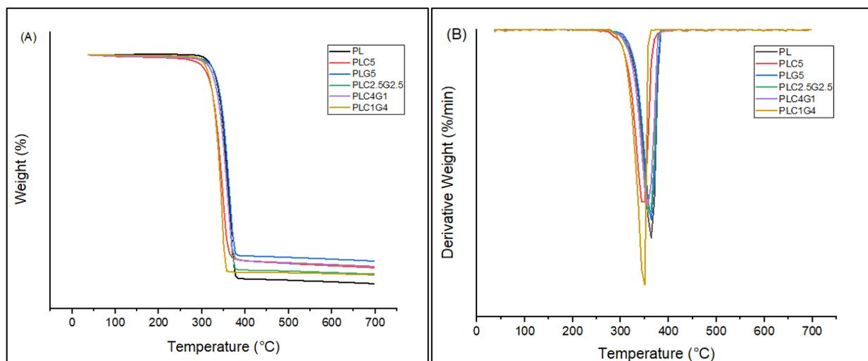
**Fig. 3:** A) TGA and B) Derivative thermogravimetric (DTG) curves for neat PLA and PLA-based biocomposite.
