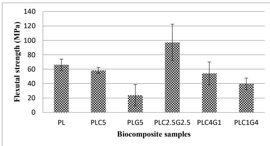
Fig. 1: Flexural strength of PLA biocomposites.
