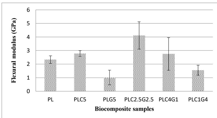
Fig. 2: Flexural modulus of PLA biocomposites.
