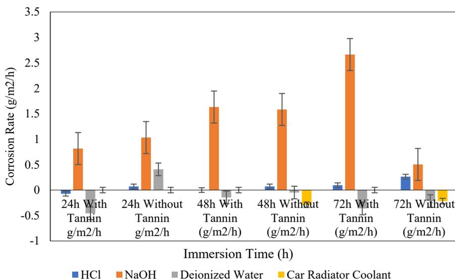
Fig. 4: Corrosion rate of aluminium substrate
