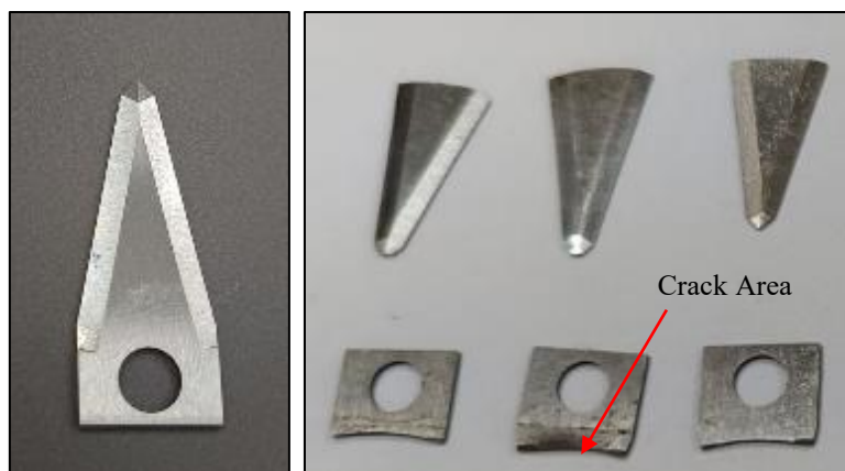
Fig. 3: Fracture of a conventional cutting blade without ultrasonic
